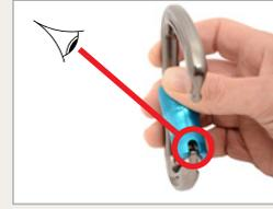
Visually inspect the gate pusher for the 'moulding line'. Look carefully at the gate pusher in your carabiner, it may be necessary to open the gate, a good light source is essential. Angling the carabiner in the light will help bring the moulding line into relief. The moulding line is visible from both sides of the gate.
